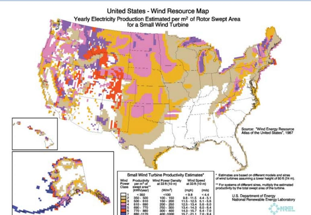
Figure 2: Energy production for small wind turbines in the United States.
