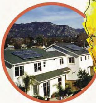
**Outstanding solar resource**—A typical home in Los Angeles needs 234 ft<sup>2</sup> of roof space to meet one-half of its typical electricity needs—using a solar power system with a conservative 12% conversion efficiency.
