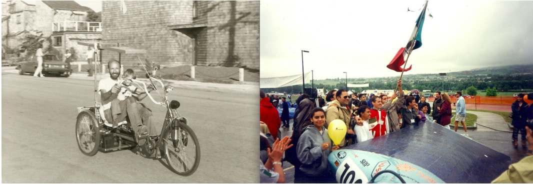
Fig. 1. (a) “The tricycle pictured here.. will travel 20 miles at a top speed of 15 miles per hour... The panel... converts sunlight directly to 35 watts of electricity...” [1] 1981 (b) Tonatiuh team at finish line, Sunrayce ‘95
